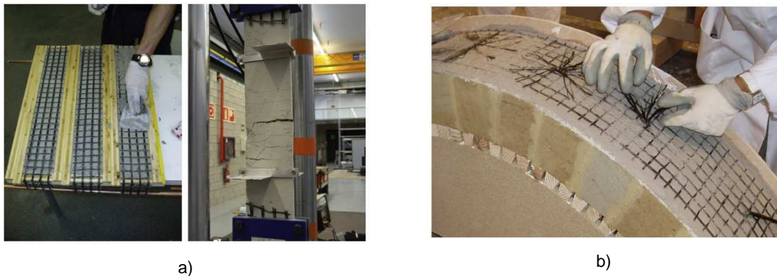
Fig. 2.13. Basalt-Textile applied to a) a specimen; b) an experimental arch [27].
