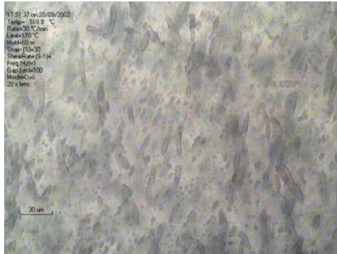
Figure 4.9 - Morphological evolution along the extruder length for the blend with 10 wt % LCP, at T=170\text{ }^{\circ}\text{C} , \gamma_0 = 0.3 (conducted using the Linkam optical shear system).
