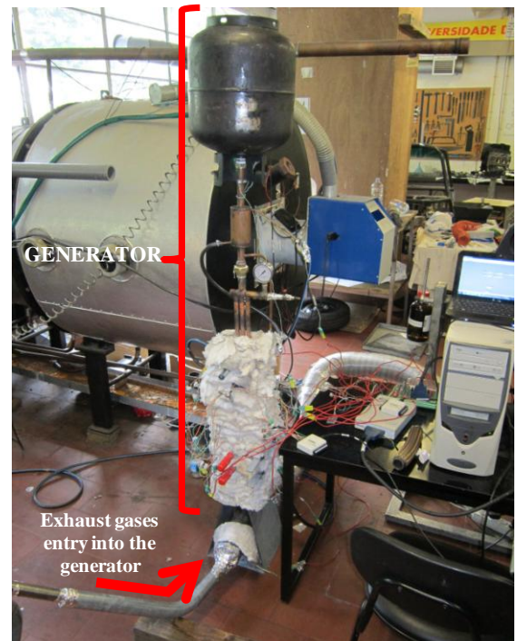
Figure 8. Apparatus connected to the exhaust of the engine
