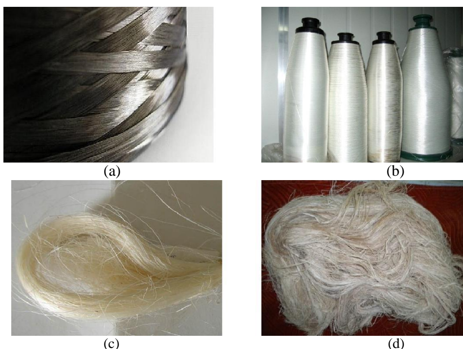
Fig 1. Example of fibers used in teh study: (a) basalt; (b) glass; (c) sisal; (d) banana
