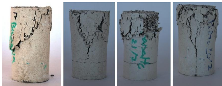
Fig. 6 Crack patterns under compression
