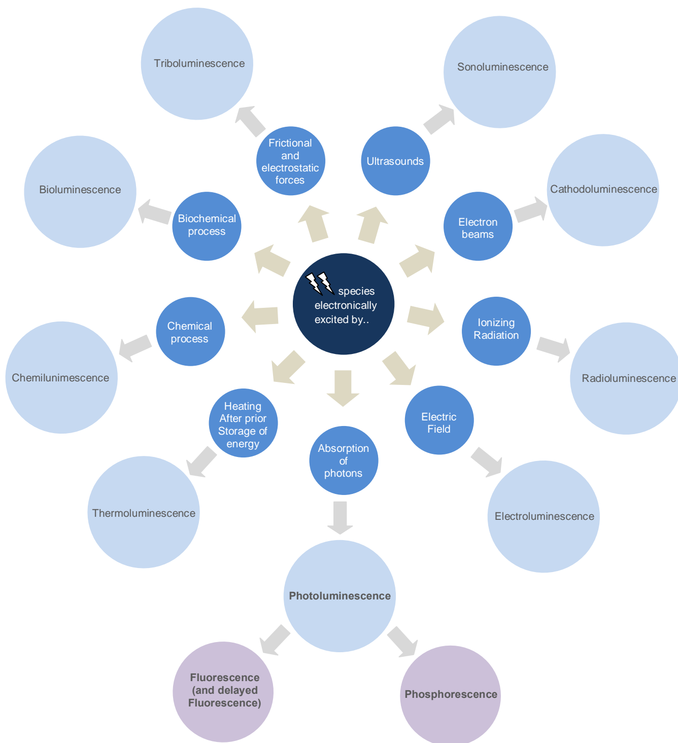
Figure 4.3. Types of luminescence processes and respective ways of molecules excitation (adapted from ref. 3).
