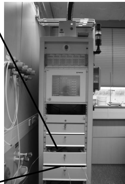
Figure 7.4: Sensor in housing connected to gas supply of the EDGaR installation.
