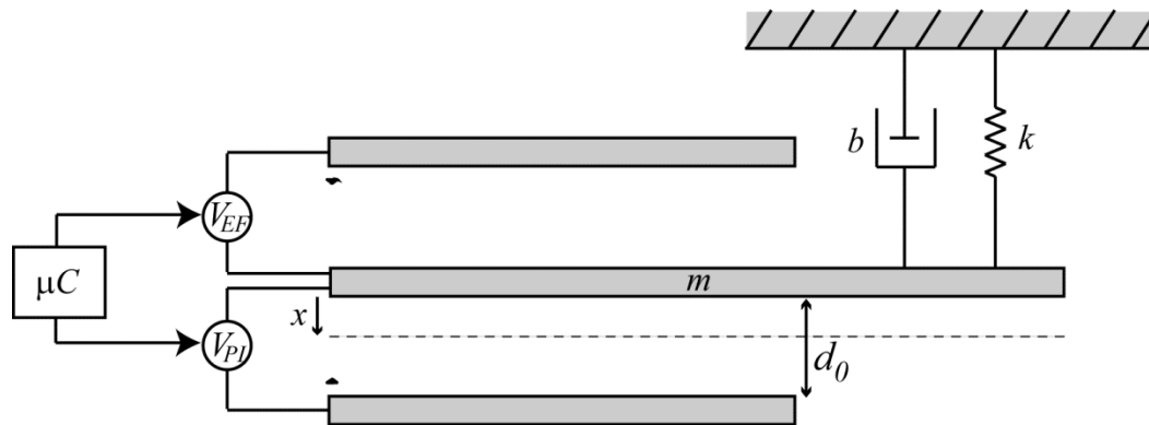
Figure 1.7: Electrostatic counter actuation of parallel-plate structure.
