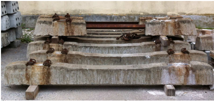
Figure 2.3: Concrete mono-block (bottom) and twin-block (top) sleepers.
