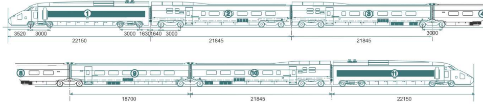
Figure 4.7: Configuration of the Ave-Alstrom high-speed train: locomotives (wagons 1 and 11), laboratory wagon (2), end wagons (3 and 10) and middle wagons (4 to 9), (Galvín and Domínguez, 2009).
