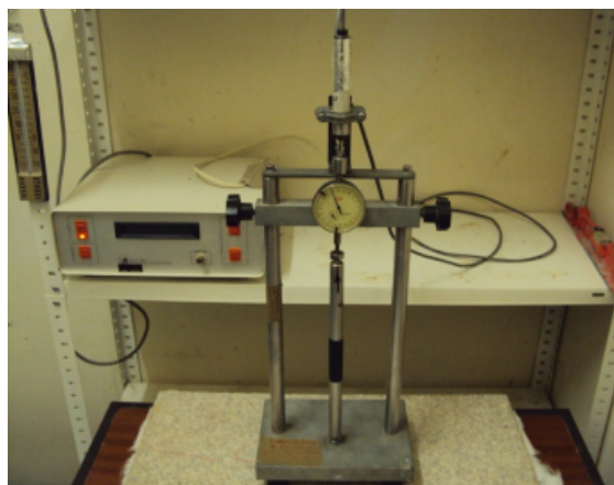
Figure 2: Measurement device method for testing mortar shrinkage.
