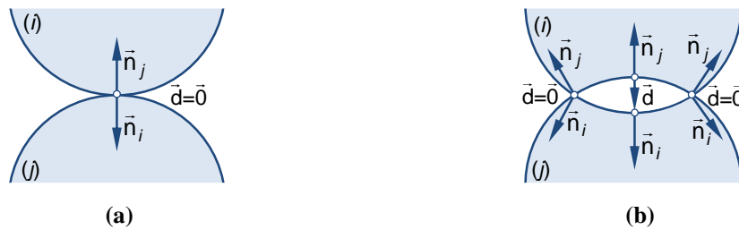
Figure 5.4 Two possible contact scenarios: (a) Contact at a single point without indentation; (b) Contact at a multiple points with indentation.
