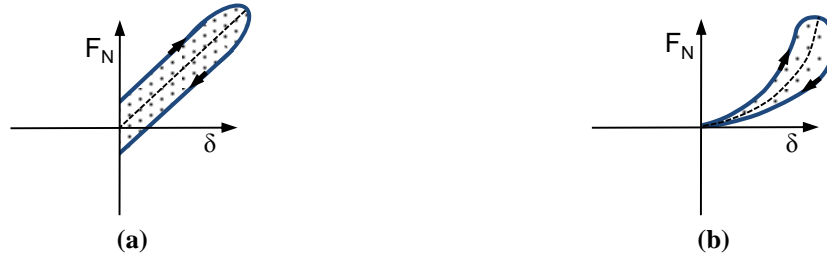
Figure 4.8 Schematic diagram of a normal contact force-indentation relation for: (a) Spring-dashpot model (e.g., Kelvin and Voigt law); (b) Nonlinear damping model (e.g., Hunt and Crossley law).
