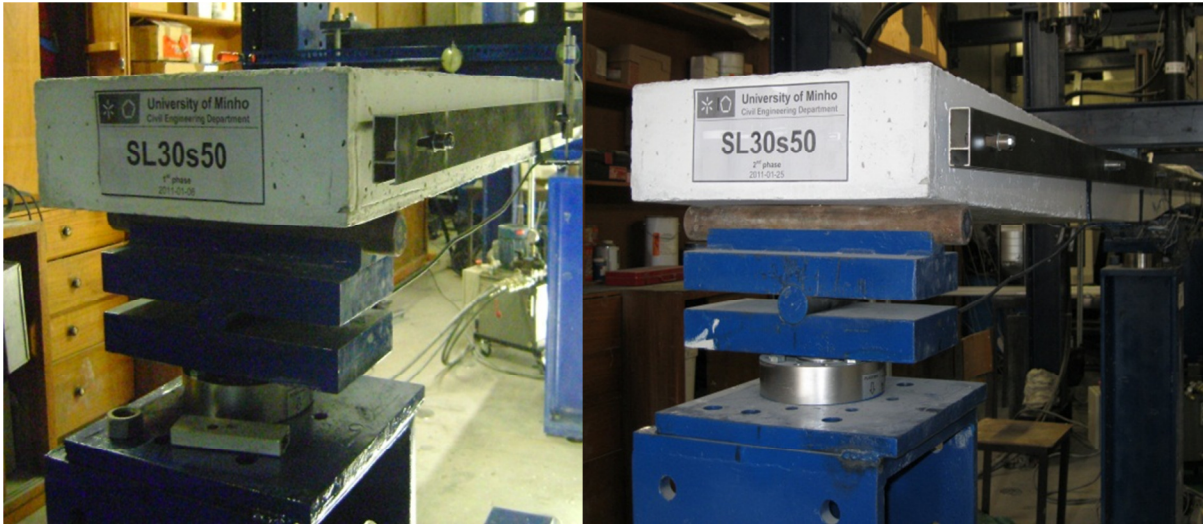
Figure 3.62: SL30s50-HS specimen before (a) and after having been tested (b).
