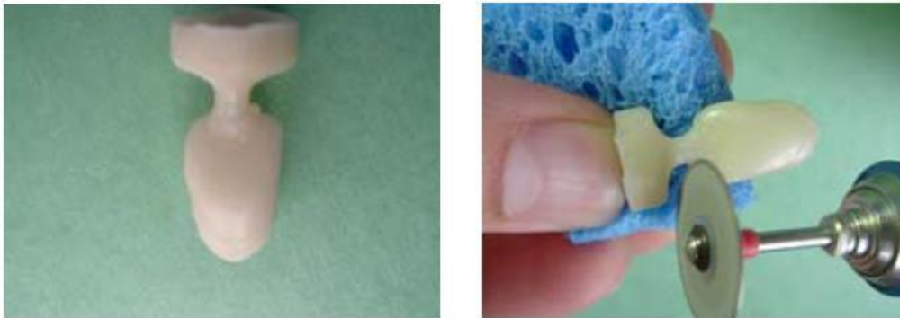
Figure 9.8. Separation of the sprue using a diamond disk.
