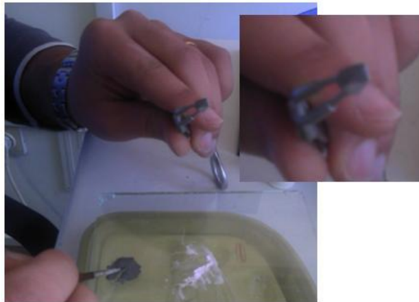
Figure 9.2. Application of the metal-ceramic composite interlayer with a brush.
