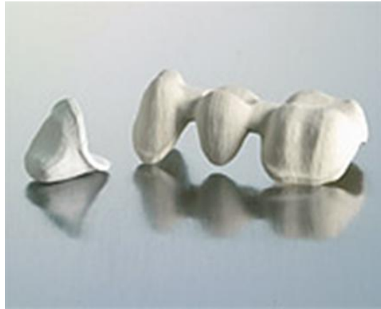
Figure 1.12. Zirconia porous structure obtained by slip-casting and after a 10 hours sintering stage at 1120°C. After it should be infiltrated by a low viscosity lanthanum glass for 4-6 hours at 1100°C to produce a dense ceramic structure (In-Ceram-Zirconia).
