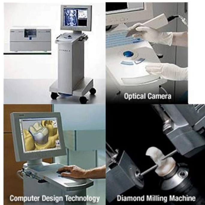
Figure 1.13. CEREC CAD-CAM system, which constructs ceramic partial dentures from machined dry-pressed ceramic blocks.
