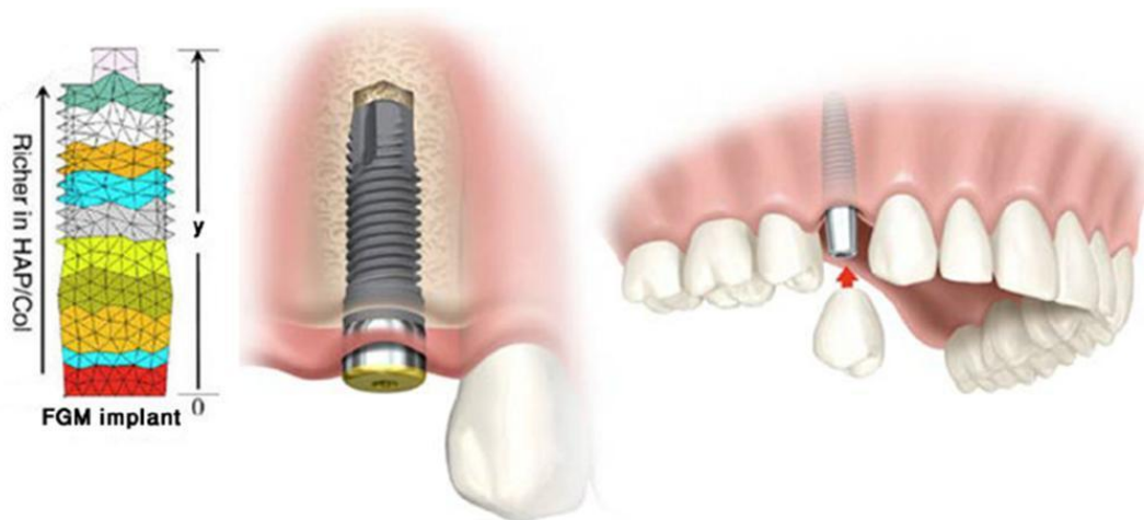
Figure 1.25. Schematic view of an FGM dental implant with graded materials composition (Sadollah and Bahreininejad, 2011).
