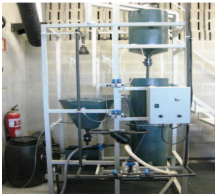
Figure 1: Overview of the pilot plant scale: a) real representation; b) SolidWorks representation
