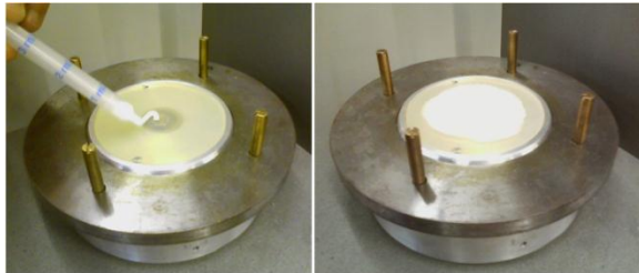
Figure 6 – Deposition of 0.5 ml of moisturizing cream
