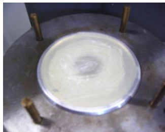
Figure 7 – A cream film applied manually to the lower support base of the silicone rubber
