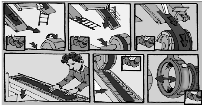
Figure 96 - Tread assembly with two breakers, cap ply and on top of it the tread. [7]
