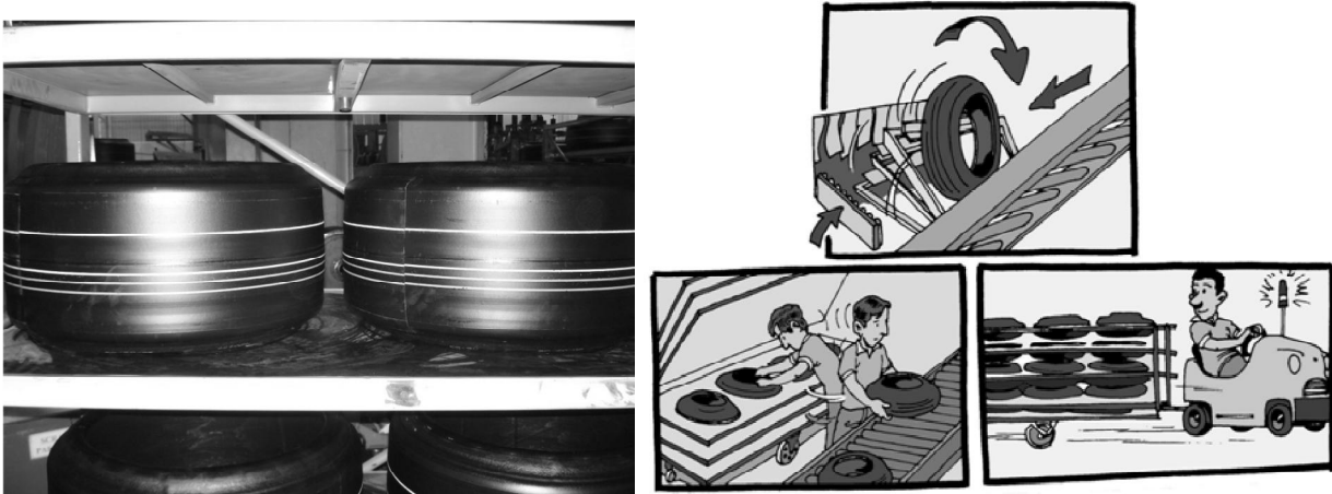
Figure 99 - green tire storage and transfer [7]
