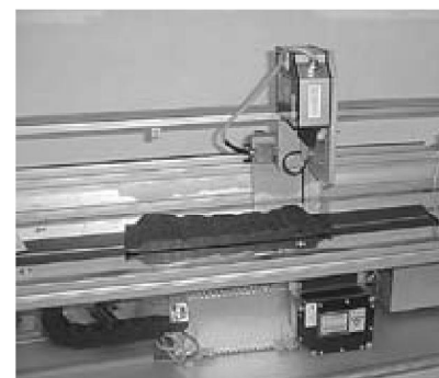
Figure 23 - The SLS5000 noncontact industrial gauging sensor is shown in a scanning frame system as it profiles extruded rubber tread.
