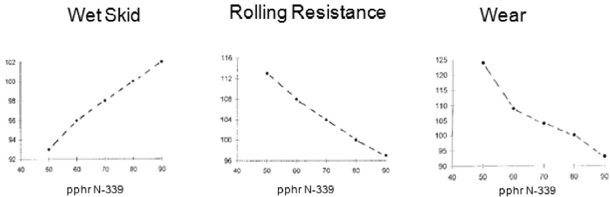
Figure 39 - Carbon black effects on wet skid, RR and wear [2]
