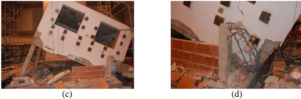
Figure 14 - Collapse (out-of-plane expulsion) of the infill walls in model 1 during the last stage: (a) outer leaf of the South wall; (b) inner leaf of the South wall; (c) North Facade after stage 4; (d) failure of a corner column of the first floor.
