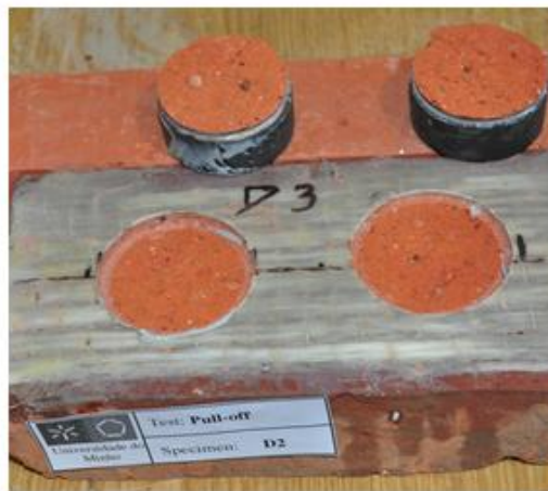
Figure 5. Typical failure mode in the specimens.
