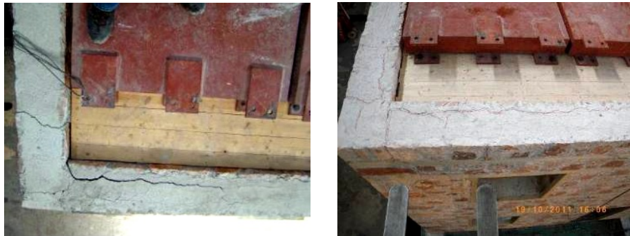
Fig. 8 Detachment of the leaves of the three-leaf masonry at the roof of the a) unreinforced (90% input signal) and b) timber-laced specimen (120% input signal)
