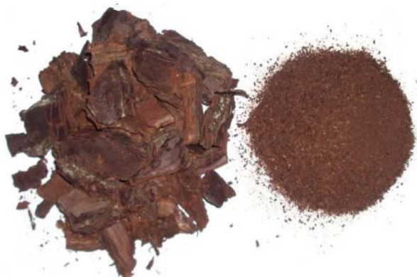
Fig 1: Pine bark sampling before and after milling
