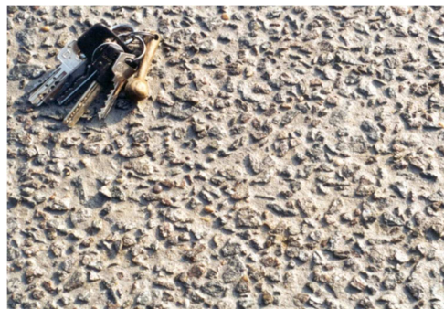
Fig. 23. A hardened two layer exposed aggregate cement concrete surface with 0/7 aggregate in the top layer.
