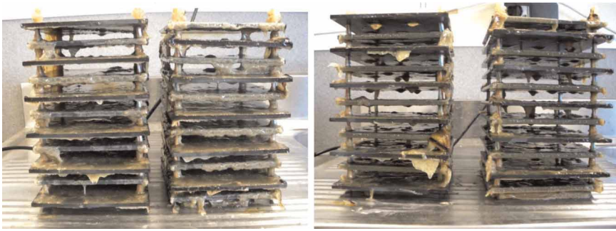
Figure 4 | Photographs of the two submodules with non-pierced plates (left) and with pierced plates (right), showing the grown biofilms on the plates and hanging from the cascades and from the holes.
