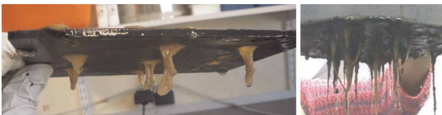
Figure 6 | Photographs showing hanging biomass: from a pierced plate of the present research (left) and from the liquid distributor of previous works using a pure strand of P. putida . Note the dimension of each formation comparing with the thumb (left) and the arm (right).
