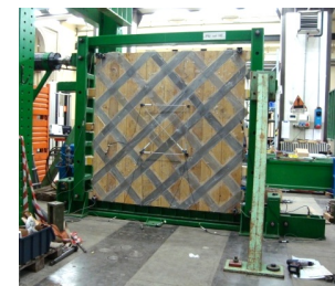
Fig. 4 Laboratory setup (hemp net specimen)
