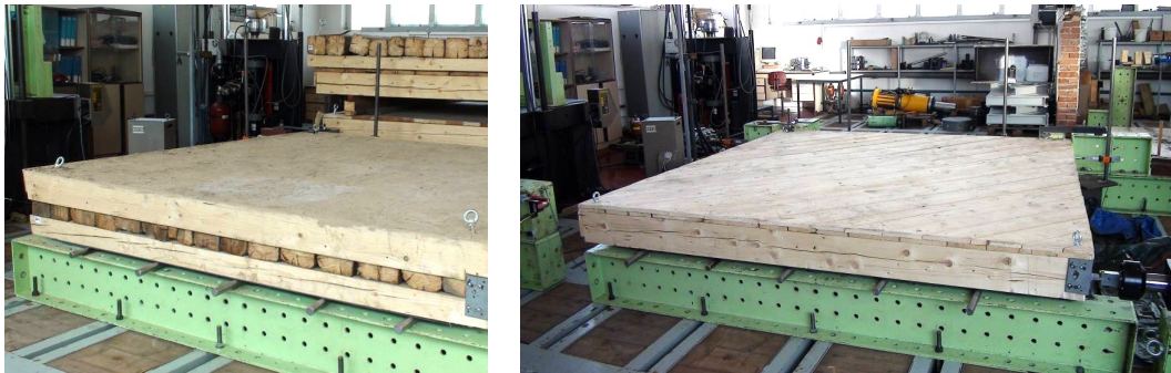
Fig. 7 Wooden ceiling with trodden earth floor (left), joist ceiling with double planking (right)
