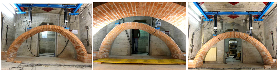
Fig. 12 Strengthened vaults at end of test: SRG-C (left), BTRM-C (center), SRP-C (right)
