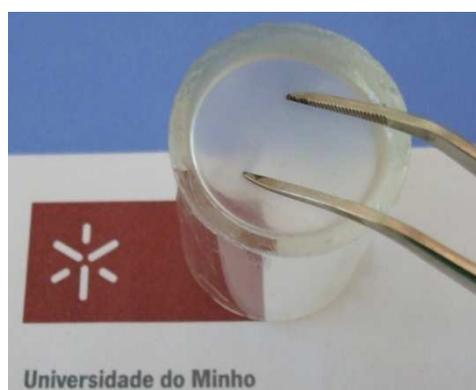
**Figura 20-** Filme do SPE  $a\text{-pEO}_{12}(\text{LiBF}_4/\text{Eu}(\text{CF}_3\text{SO}_3)_3)$
