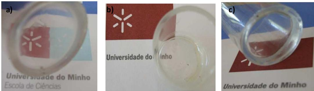
**Figura 28-** Filmes de SPEs baseados no sistema (a-PEO<sub>x%</sub>/pTMC<sub>y%</sub>)<sub>n</sub>LiX: X<sup>-</sup>=ClO<sub>4</sub><sup>-</sup>: **a)** X%=95%, Y%=5%, n=8; **b)** X%=90%, Y%=10%, n=12; **c)** X%=15%, Y%=85%, n=12.
