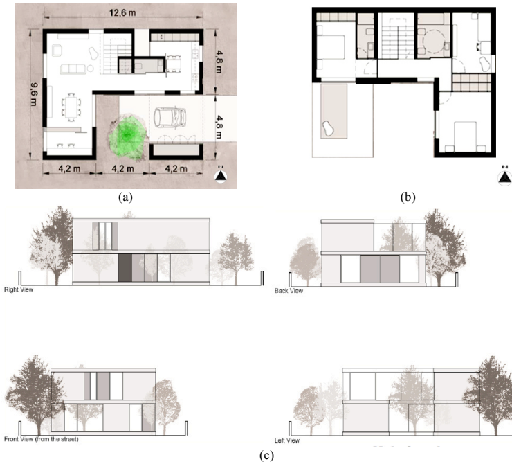
Figure 1 – Single family-house used as case study. Plan view of the ground floor (a) and first floor and the four lateral views
