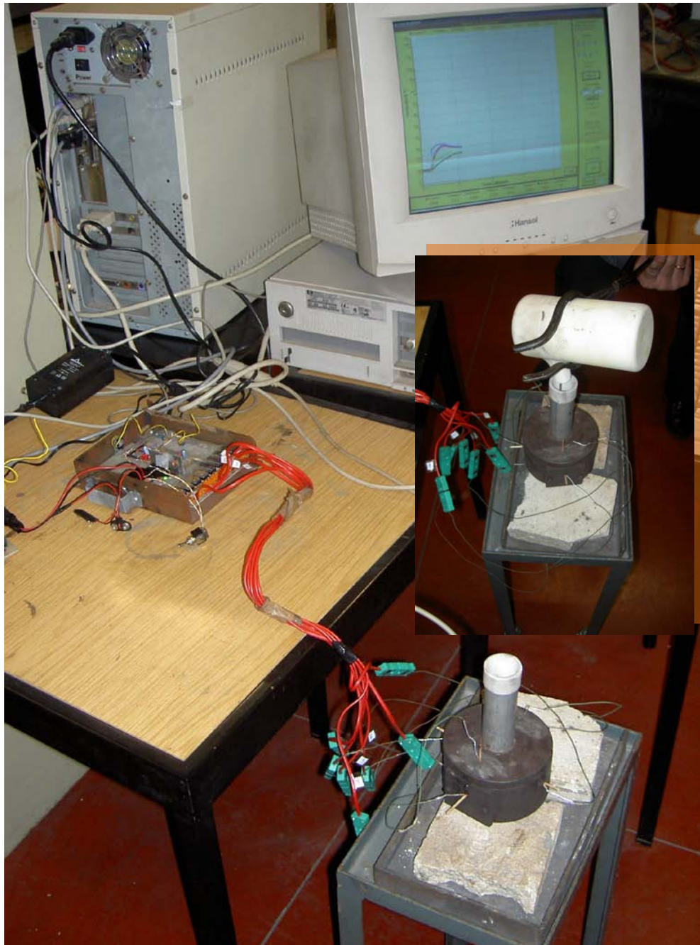
Figure 3.10 - Temperature acquisition system during gravity casting
