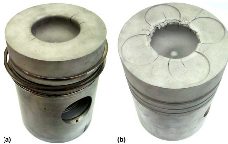
Figure 1.13 - Train engine pistons with damaged head: (a) piston 1; (b) piston. [5]
