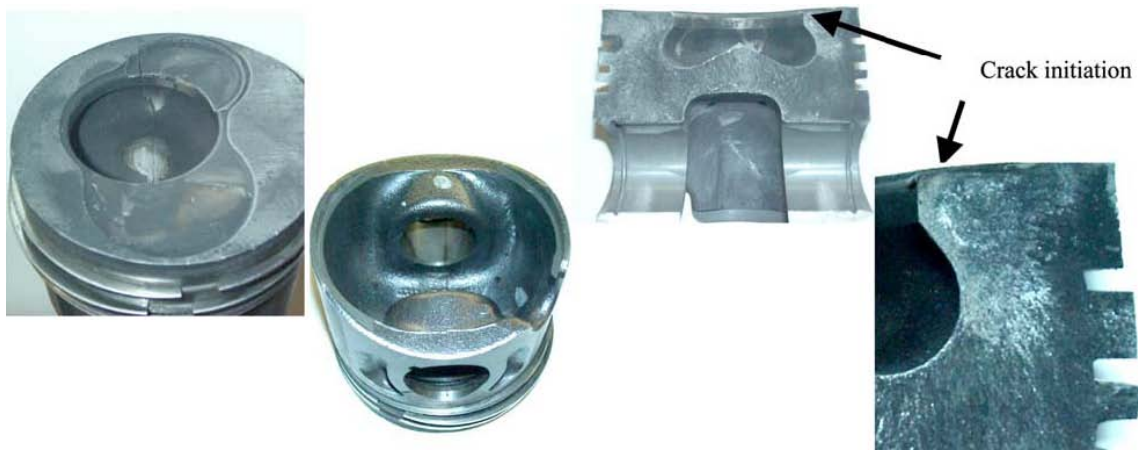
Figure 1.6 - Diesel engine piston with a crack from one side of the pin hole to the other pin hole going through the head of the piston.
