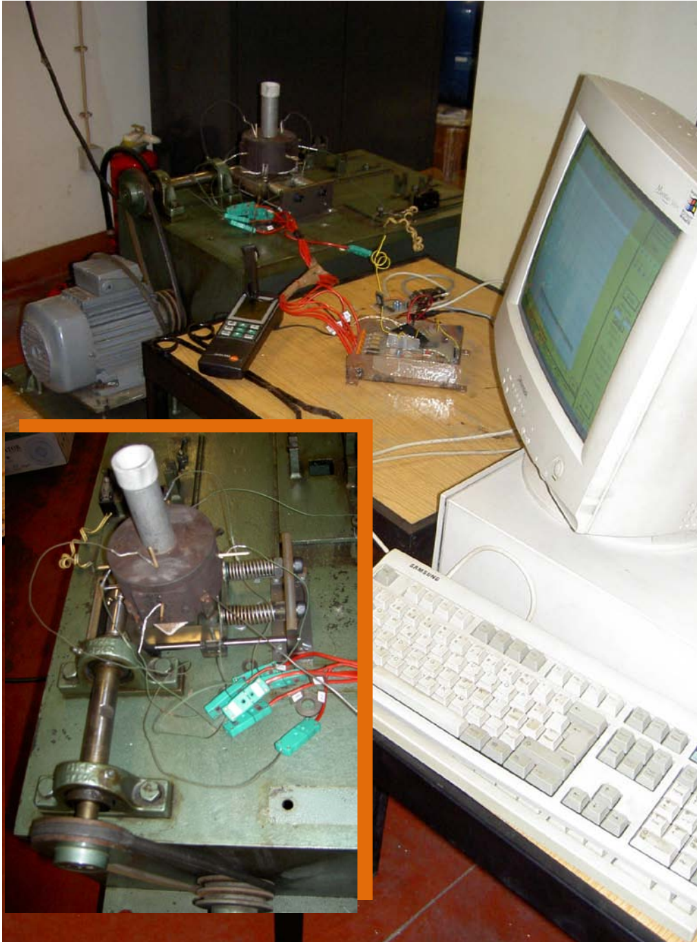
Figure 3.9 - Temperature acquisition during vibrating gravity casting
