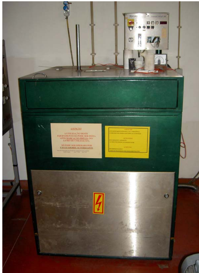
Figure 3.1 - High frequency induction furnace: Titancast 700 mP Vac, from Linn High Term, Germany (Foundry Laboratory – Minho University)
