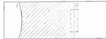
\alpha_c \alpha = 0, 2\pi \alpha_g (max. gap) (c) commonly adopted boundary conditions: rupture - pressure and pressure gradients equal to zero at \alpha = \alpha_c reformation - pressure equal to zero at \alpha = \alpha_g
