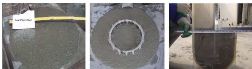
Fig. 1. Tests of workability of SCC with 40 kg/m 3 steel fibre.
