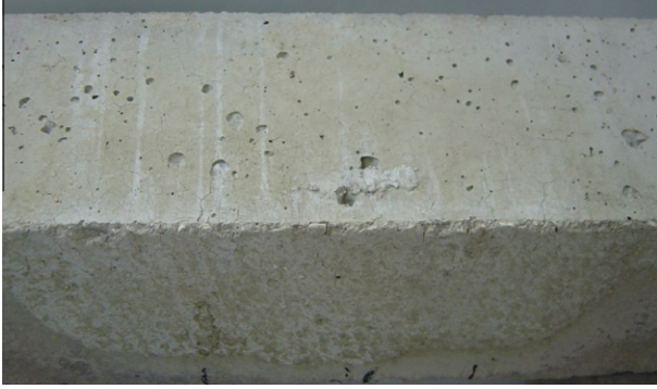
Fig. 14. No spalling of beam PP2 after 600 °C.
