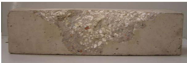
Fig. 10. Spalling of SCHPC beams without fibres after 600 °C.
