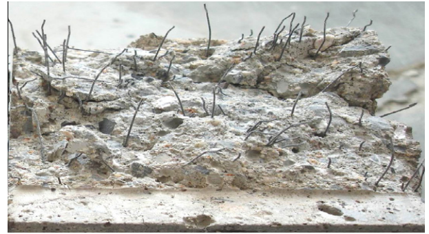
Fig. 13a. Failure pattern of SF55 after 600 °C.
