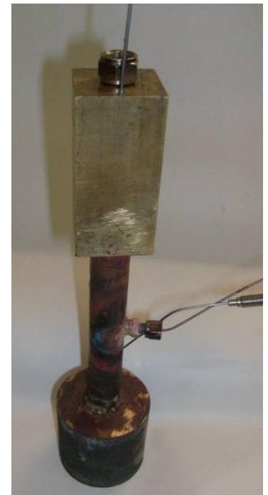
Figure 10 - (a) Outline and (b) photograph of Heat Pipe setup, with 20 L cylinder tank for VCHP operation and thermoelectric modules. (c) Detail of the bare HP without the tank nor the TEGs attached
