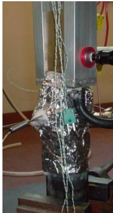
Figure 10 - (a) Outline and (b) photograph of Heat Pipe setup, with 20 L cylinder tank for VCHP operation and thermoelectric modules. (c) Detail of the bare HP without the tank nor the TEGs attached
