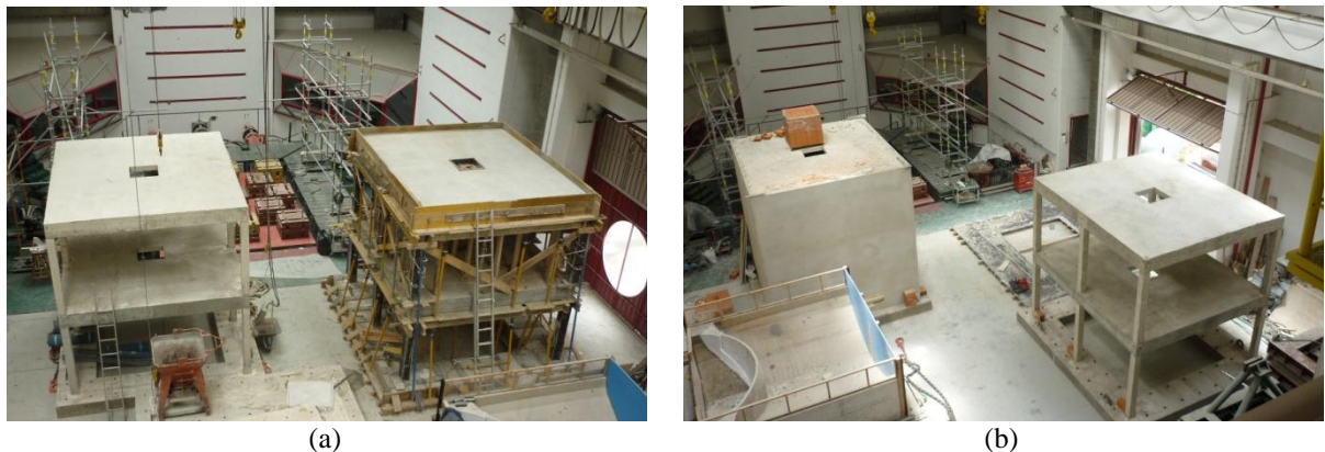
Figure 3: Construction of models 1 and 2: (a) concrete structure; (b) infill walls.
