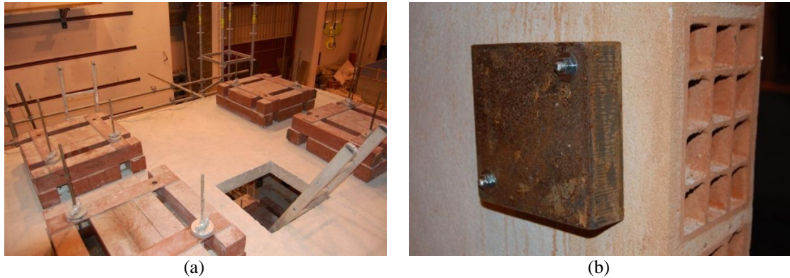
Figure 6: Additional masses: (a) for the concrete structure and floor loads; (b) for the infill masonry walls.
