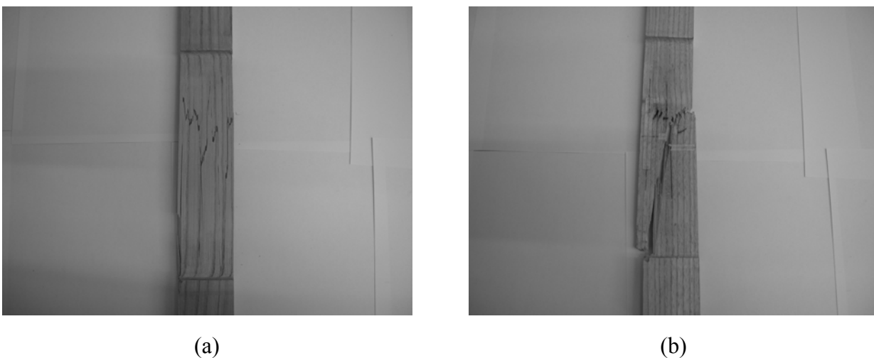
Figure 6.8 – Typical failure patterns observed: (a) splinter, and (b) shear and tension failure.
