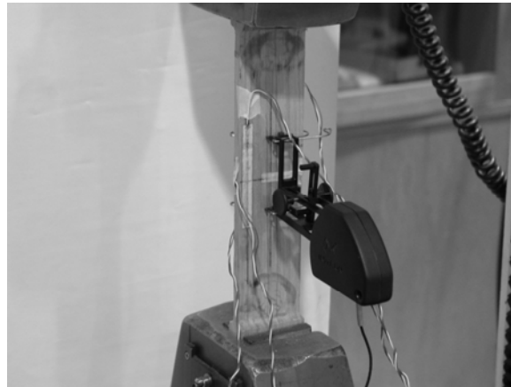
Figure 6.5 – Bonded strain gauges and mechanical strain gauge.
