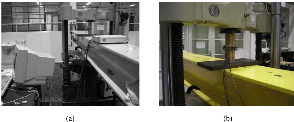
Figure 5.3 – Compression testing: (a) general view, and (b) test piece under testing.
