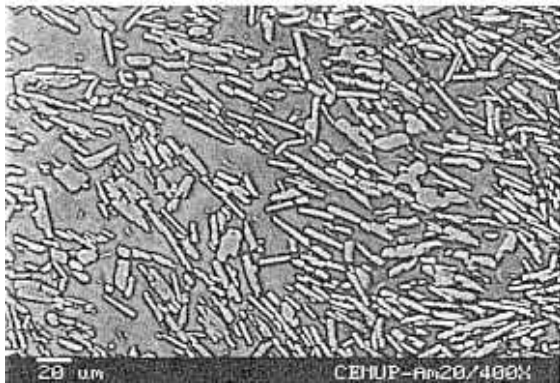
Fig. 12 Microstructure of a sample melted and cooled in a graphite crucible
