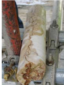
Fig. 3.41 Masonry specimen extracted from the arch bridge
