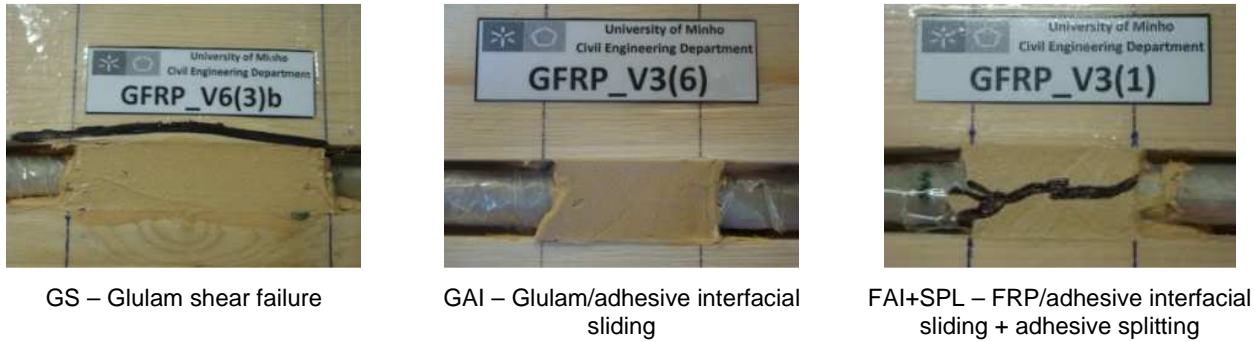
Figure 7 – Typical failure modes obtained
