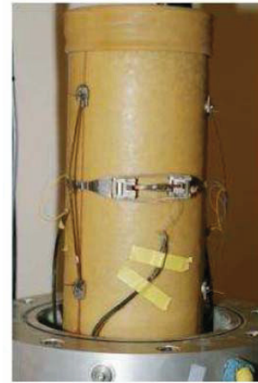
Figure 1: Triaxial sample with vertical and radial LDT transducers
