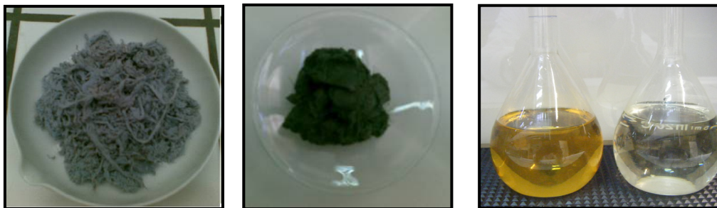
Figure 1 – Leather waste a) Wet-blue scrapings and products obtained after applying the procedure: b) Chromium rich cake; c) Raw hydrolysate and d) Organic fertilizer
