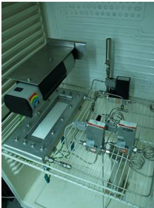
Figure 1 – Experimental set-up for studying the NO x photocatalysis. This unit is suitable for reproducing the operating conditions described in the relevant standard ISO 22197-1:2007(E).
