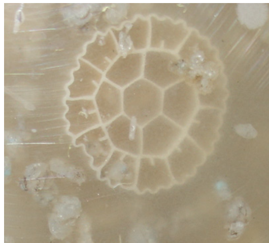
Figure 2. Image of one Kaldnes K-3 ring and some particles of rough plastic support
