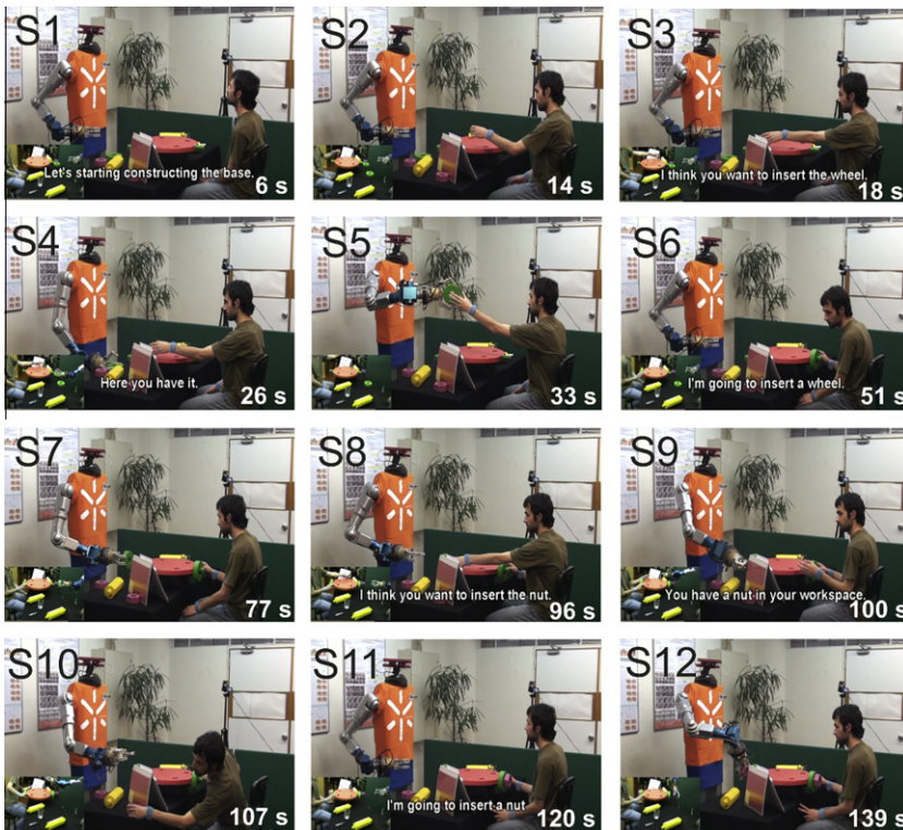
Fig. 8. Video snapshots that illustrate a scenario where the same observed action may have different interpretations, depending on the context in which it occurs, and thus lead to different action selection.
