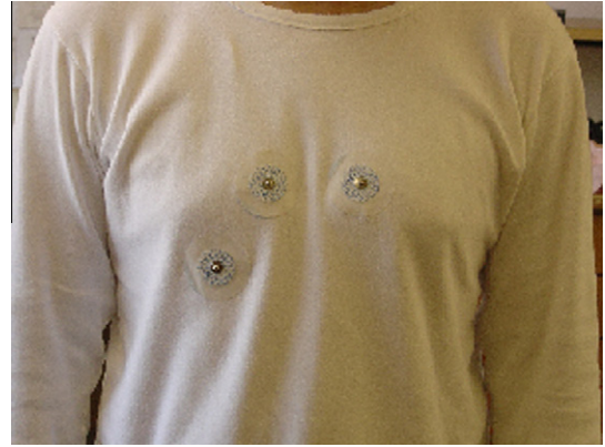
Fig. 11. A photo of the patient wearing a electronic shirt ready to plug RF modules.
