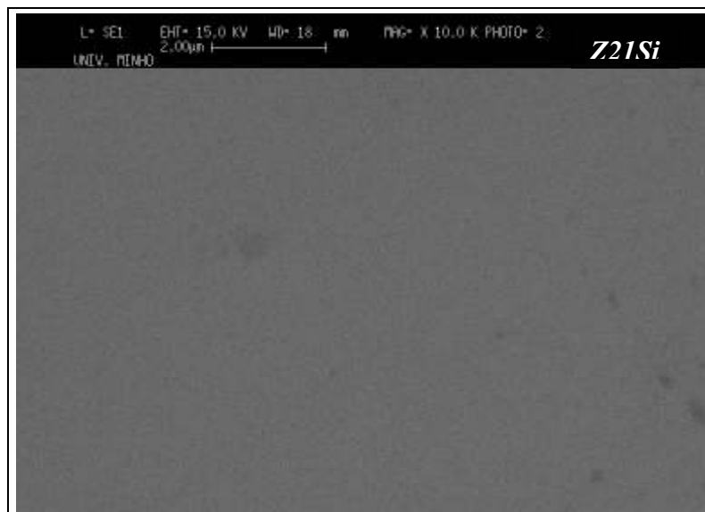
Fig.3.6 – Top view surface picture of sample Z21Si, obtained by SEM. Darkest dots on the picture were not possible to identify. Some of them may possibly be small areas with higher Ge concentration.
