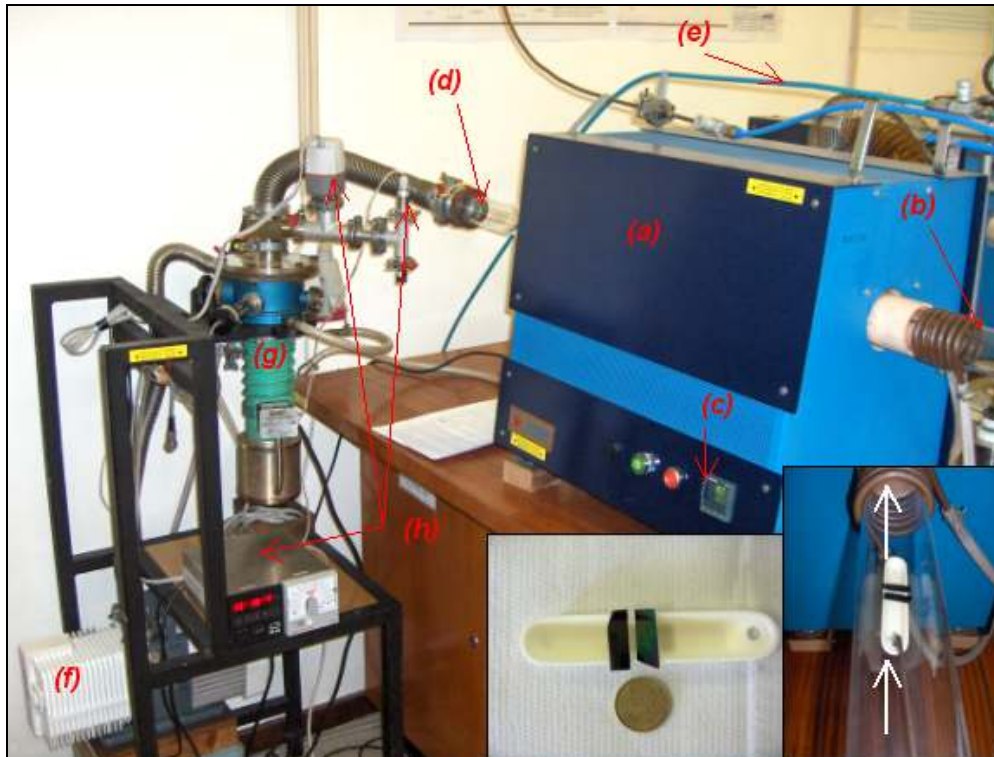
Fig.2.7 – Annealing system used: (a) oven, (b) thermocouple, (c) temperature controller, (d) quartz tube, (e) gas lines, (f) rotary pump, (g) diffusion pump, and (h) pressure gauges.
