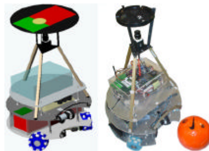
Fig. 2. CAD drawing of the complete robot and final real robot
