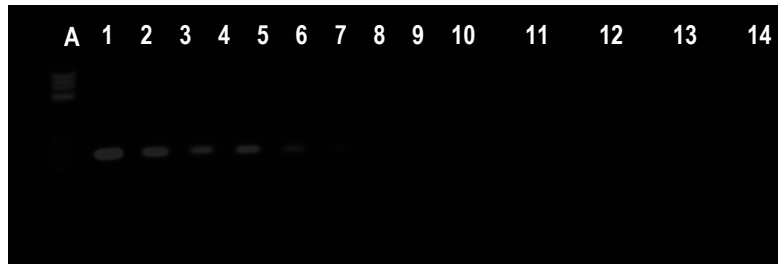
Figure 6.4: Representative photograph of the electrophoresis gels reporting the results of the detected genes by PCR. This gel shows the results obtained for the IL-10 gene on the intramuscularly implanted SPCL scaffolds (1 to 6), and on the subcutaneously implanted SPCL scaffolds (7 to 13). Line 14 is the negative control and A is the cDNA marker.
